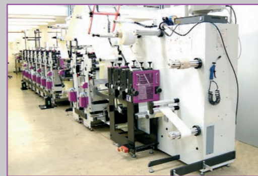
K2, 6 colour 400mm web 3 Series flexo film/label press
