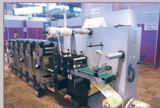
K2, 6 colour 400mm web 3 Series flexo film/label press
